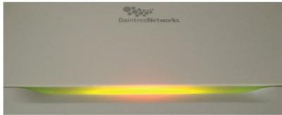
2. The WAC connects to the SC within 2 minutes of establishing an internet connection. The LED state will be solid green, as shown.
